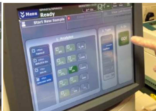
6a) Select "Glucose only" (b) check only 'glu' is highlighted then press "Go" (c) use scanner to scan your barcode
