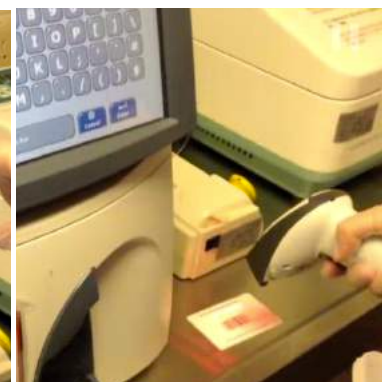
6a) Select "Glucose only" (b) check only 'glu' is highlighted then press "Go" (c) use scanner to scan your barcode
