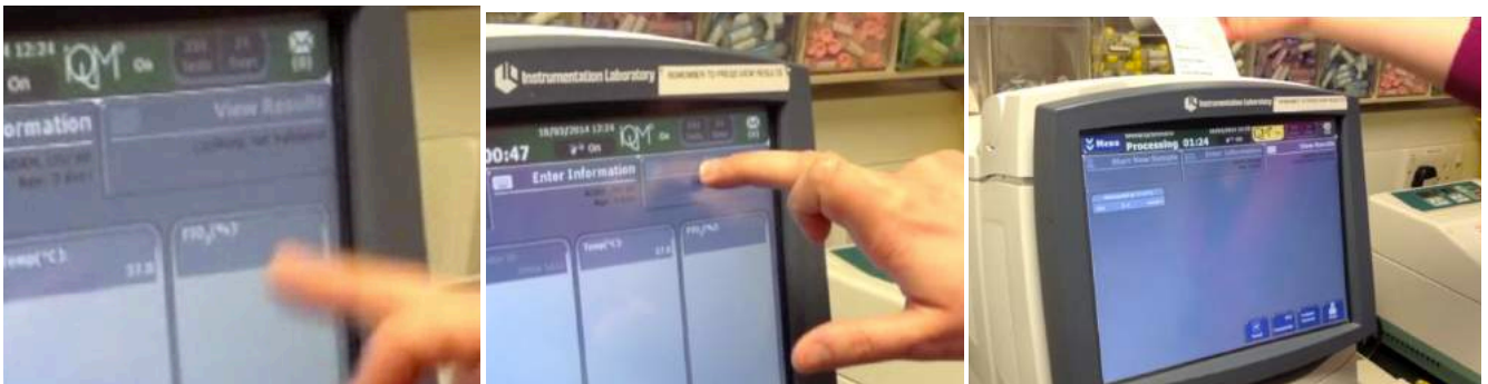
(m) once you've entered details you must click "View results" (n) results will then print out automatically when ready
