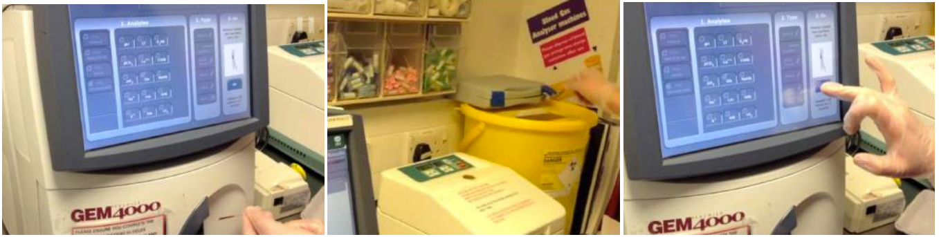
(g) once it's finished and beeps remove sample (h) dispose of used gas tube into sharps bin (i) then press "OK"
