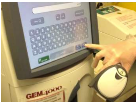
(d) press "Enter" (e) put capillary gas tube into the receiver (f) press "OK" and watch the machine aspirate the blood
